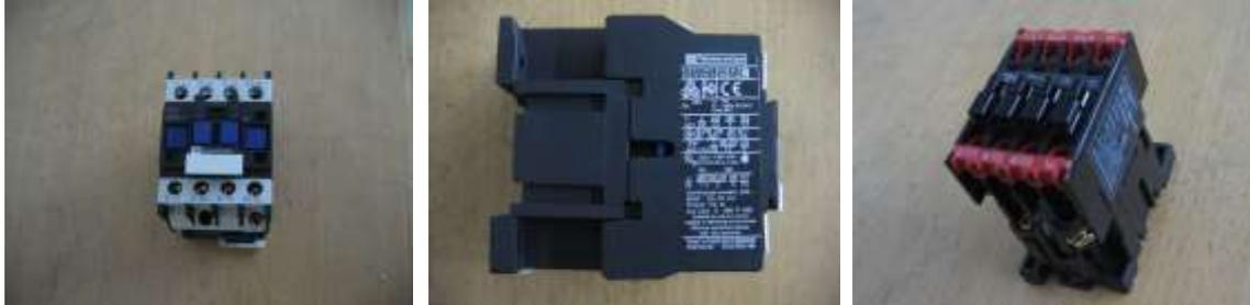
The function of the AC electromagnetic contactor is to protect the start-up assemblies of the motor. If it has been damaged, the following will occur:
