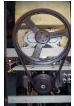
stop and there through not rotate; if the strap is too tight, the motor resistance and current will increase and the control system will reach the value when the cooling cycle should stop to early. This will result in that the machine will stop before the cooling cycle is complete or even before the compressor has started; Since the work load on the motor is too big, the right rotating speed can not be reached and may cause increase in noise.
